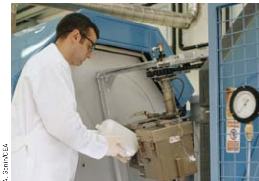
Facility, installed at CEA's Le Ripault Center (Indre-et-Loire département ), for the rotomolding of plastic liners for hydrogen-storage tanks. The mold rotates over 3 dimensions, inside an oven at 350 °C.
