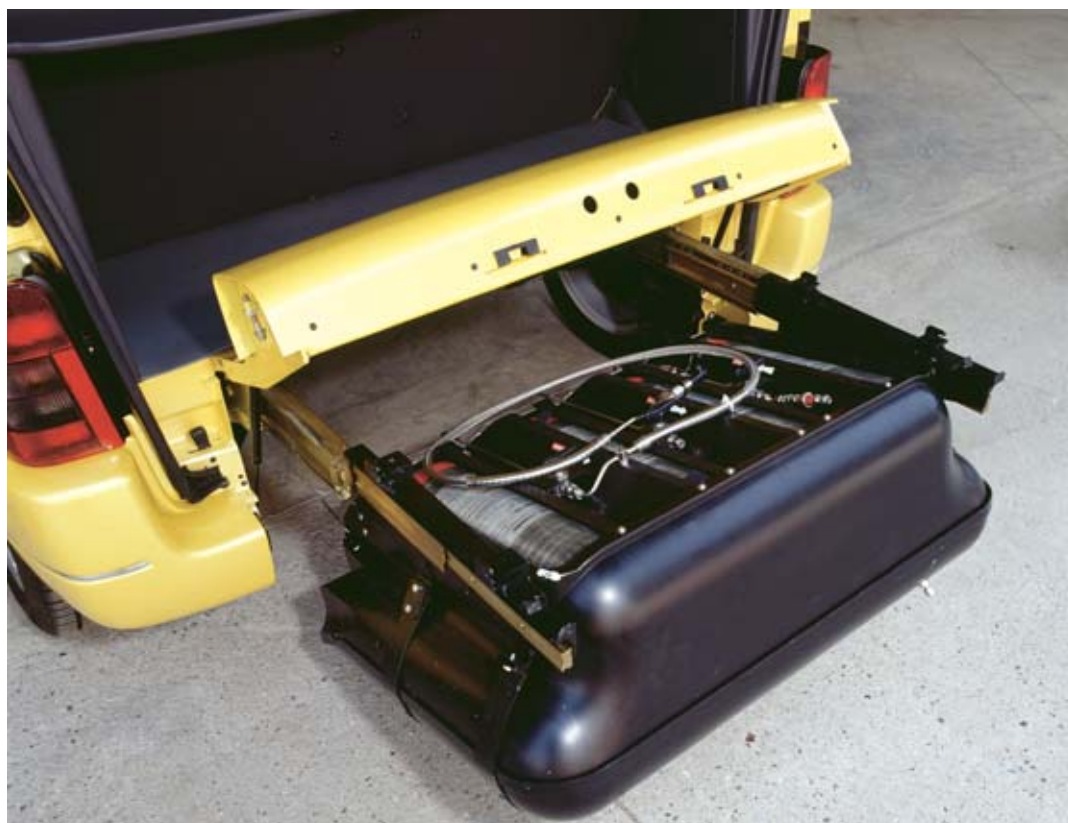
High-pressure hydrogen tank rack of the prototype TaxiPac fuel-cell vehicle, based on a Peugeot Partner chassis, as shown in 2001.
