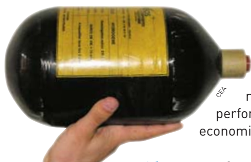
All-polymer 3-liter tank developed under the aegis of the Physe Program.
