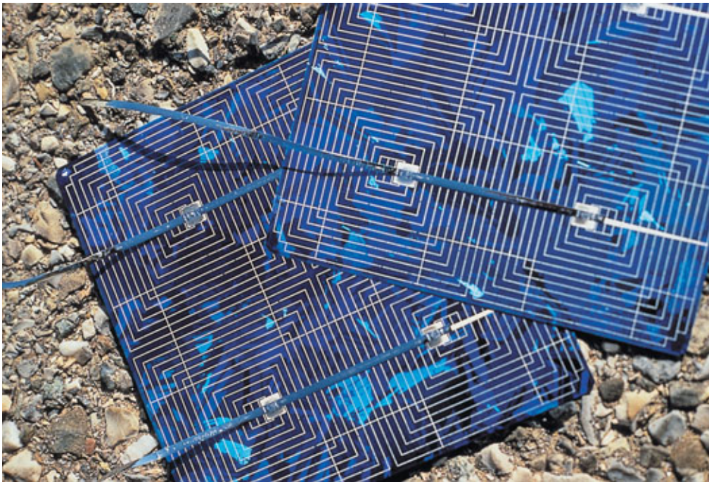
Photovoltaic cells made of polycrystalline silicon tested at the CEA by the Genec in Cadarache (Bouches-du-Rhône).
