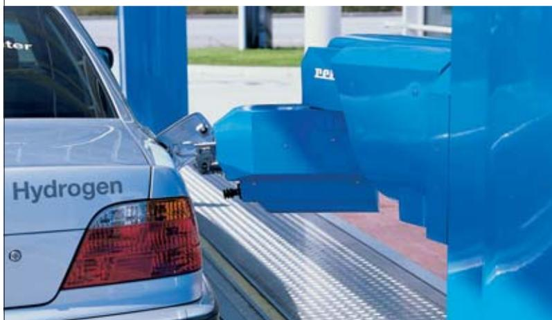
Robot-operated liquid-hydrogen filling station at Munich Airport.
