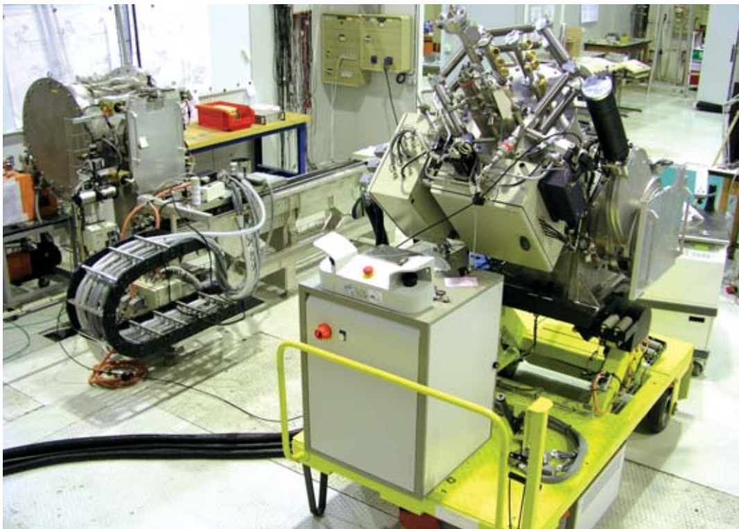
Prototype cryogenic-target carrier (CPC) in use, as a collaboration between CEA/Grenoble (Low Temperatures Service) and CESTA (Power Lasers Department). This item, which was delivered in 2002, enabled validation of the cryogenic pincer's thermal-regulation performance. Mechanical performance (positioning accuracy and loading of a target in vacuum, in cold conditions, and in fully-automatic mode) is currently being demonstrated.
