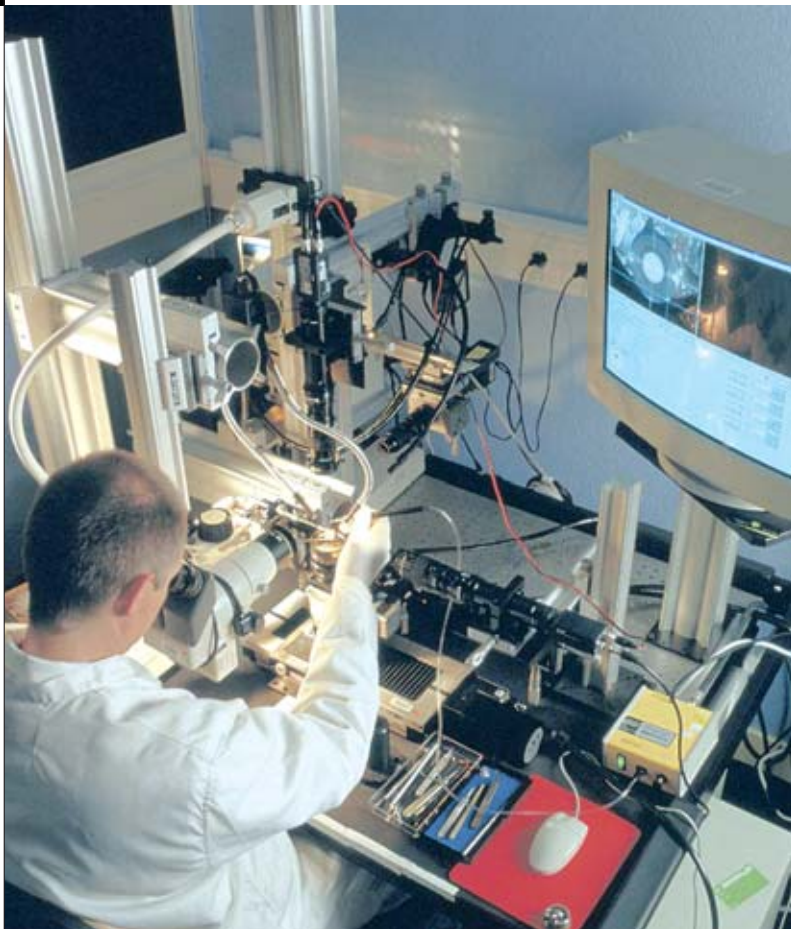
Assembly rig, at CEA's CESTA Center, for the target components coming from CEA's Valduc Center being readied for LIL and the coming LMJ. Adhesive bonding is effected by hand under visual control through a binocular magnifier, and two cameras allow onscreen visualization.
