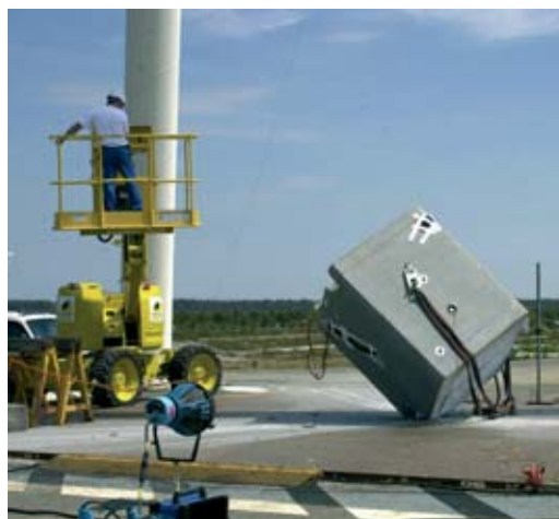
Drop test, from a height of 6 m, carried out at CEA/Cesta, with a concrete container demonstrator (common to long-term storage and disposal operations), designed to hold 4 bitumen drum primary packages. The lid remained integral with the container body, and main damage was restricted to the impact area.
