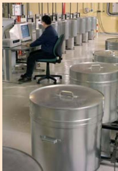
Trial platform for durability tests for metallic materials subjected to a temperature environment. The trials, initiated in 2002, have the aim of monitoring the evolution of properties over time.
