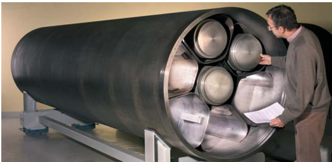
Storage container demonstrator, with the ability to hold 7 UOX assemblies (see Figure 3).
