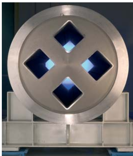
Disposal containers, compatible with storage operations (compatibility being ensured by presence of a canister), for 4 fuel assembly canisters). Their weight reaches 45 tonnes.
