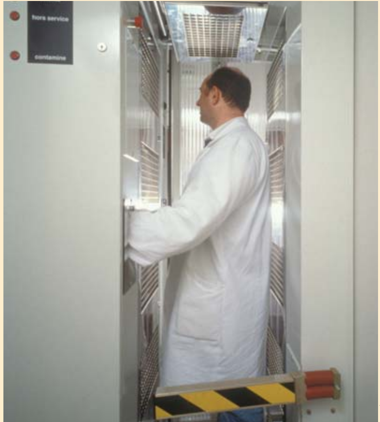
Passing through a detector frame for individual contamination at the exit from a controlled area – here the Osiris reactor at CEA Saclay Centre – is a regulatory obligation.
