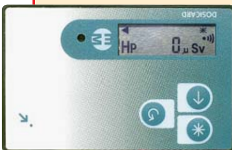
Dosicard dosimeter for real-time dosimetric monitoring.
