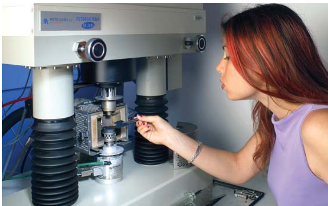
Mechanical analyzer, used to investigate the static and dynamic response of polymer membranes subjected to compression, shear or stretching stresses.
