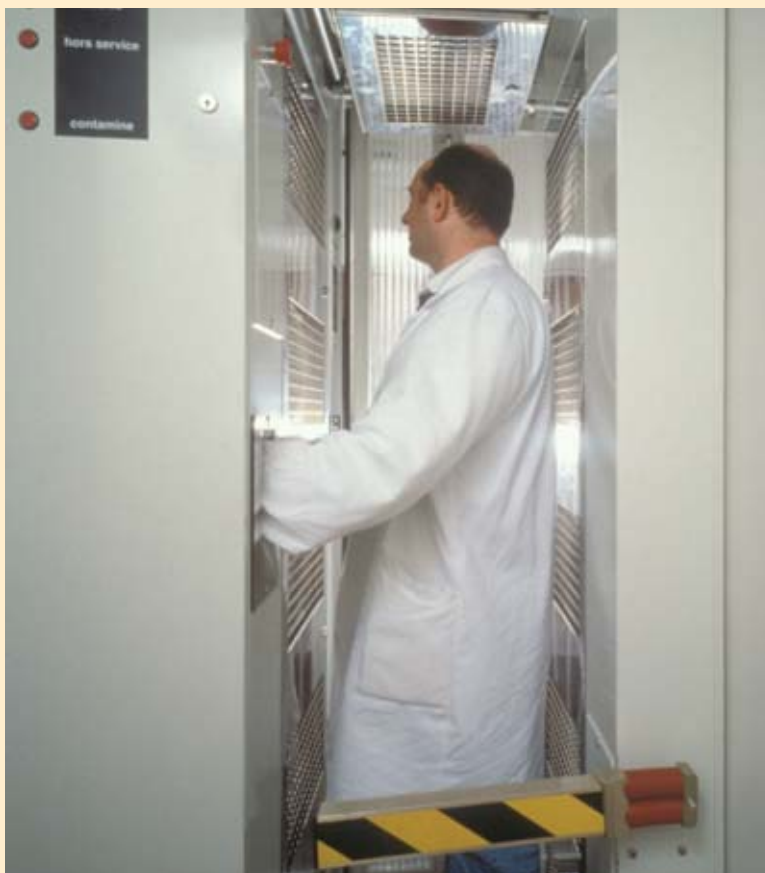
Passing through a detector frame for individual contamination at the exit from a controlled area – here the Osiris reactor at CEA Saclay Centre – is a regulatory obligation.
