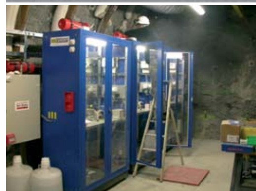
DIR experiments, carried out in the experiment niche, at – 445 m, of ANDRA's Underground Research Laboratory, at Bure (Meuse–Haute-Marne départements). Top, the experiment design selected, with injection of tracing agents at the bottom of a borehole. Bottom, experiment cabinets, in which sampling and in situ monitoring are carried out, for the experiments currently conducted in the experiment niche.
