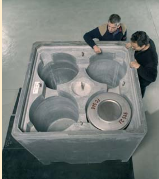
CEA design study for a common container for the long-term storage and disposal of long-lived, intermediate-level waste.
