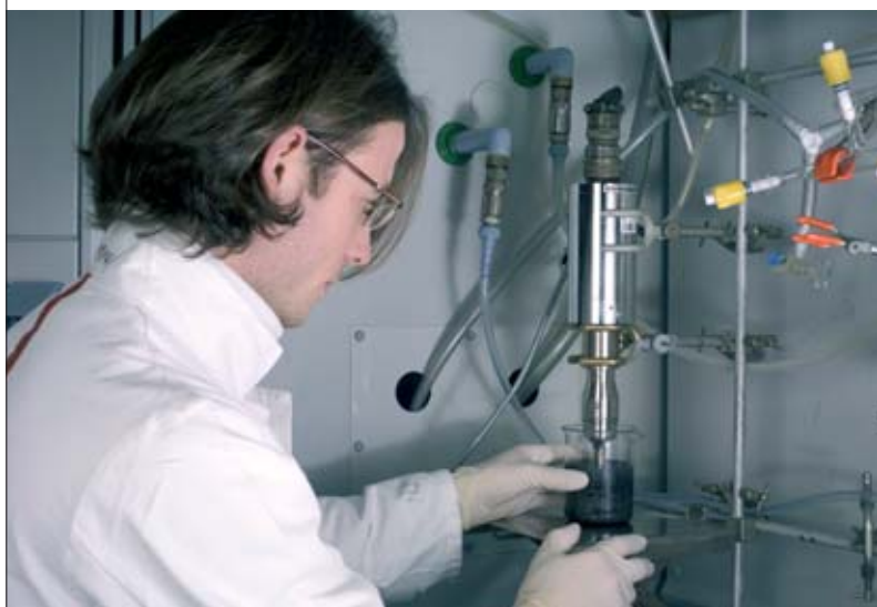
After mixing and stirring with a detergent, the carbon nanotubes are dispersed by ultrasonication to form stable suspensions.
