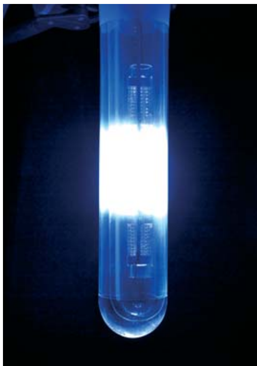
Polymerization of rings around carbon nanotubes by ultraviolet light irradiation to make them rigid.
