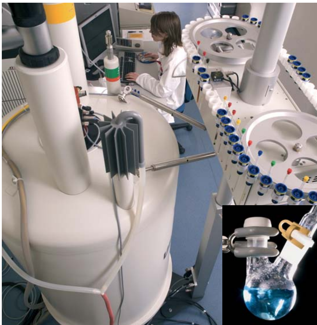
After chemical synthesis in glass round-bottomed flasks the detergents (lipids) are characterized by nuclear magnetic resonance. They are then mixed with the carbon nanotubes.
