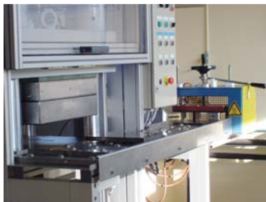
Extrusion-compression machine for fast molding of thermoplastic composites.
