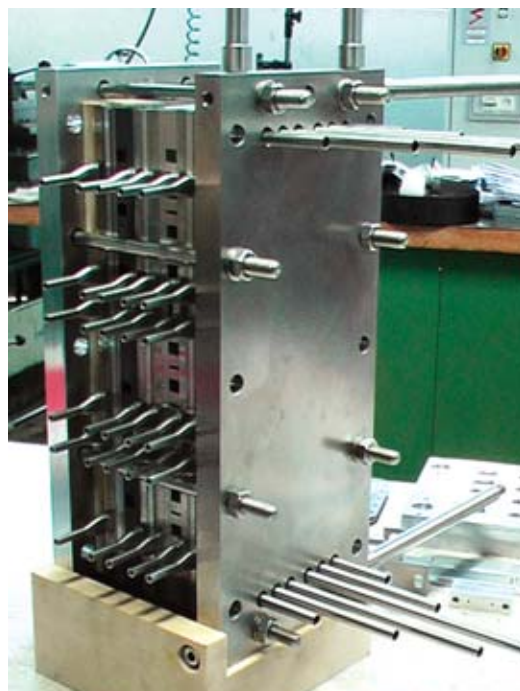
CEPACPOR stack, comprising three 225-cm 2 cells with metal-foam distributors, fitted with current-density measuring probes.
