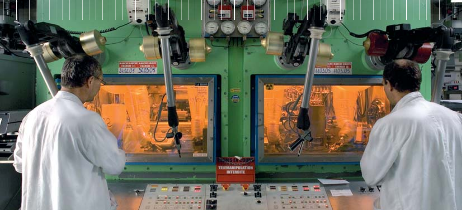
Shielded cells L6–L7 in the Atalante facility, at CEA's Marcoule Center, where preparation is carried out of pellets or targets bearing fission products, for the investigation of in-reactor transmutation.
