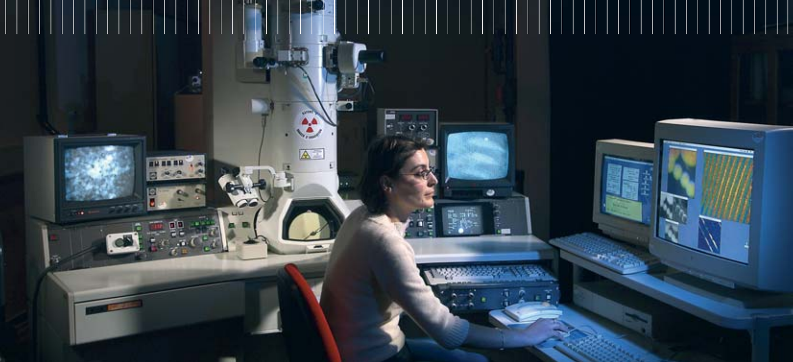
Transmission electron microscope (JEOL 300 keV) installed at CEA/Grenoble. Its point resolution is close to 0.17 nanometre.
