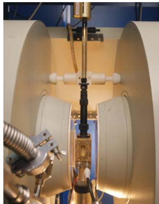
Positioning a sample for electronic paramagnetic resonance (EPR) investigation of the Mn 4 Ca complex of photosystem II. The sample is held in the EPR spectrometer at a temperature of - 269 °C, the temperature of liquid helium.
