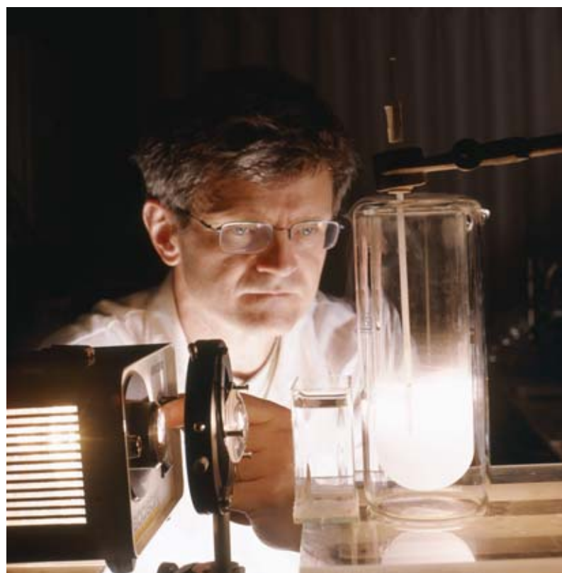
Illumination of a sample of photosystem II, the oxygen-evolving enzyme. Use of low temperature allows trapping of an intermediate state of the photochemical reaction.
