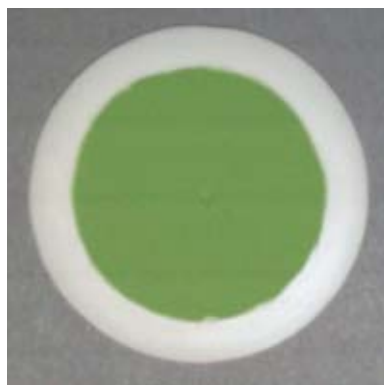
Left, composite anode in nickel oxide–yttria-stabilized zirconia, spray-deposited onto an yttria-stabilized zirconia supporting electrolyte. The nickel oxide will undergo in-situ reduction. Right, strontium-doped lanthanum-manganite cathode, spray-deposited onto an yttria-stabilized zirconia supporting electrolyte.
