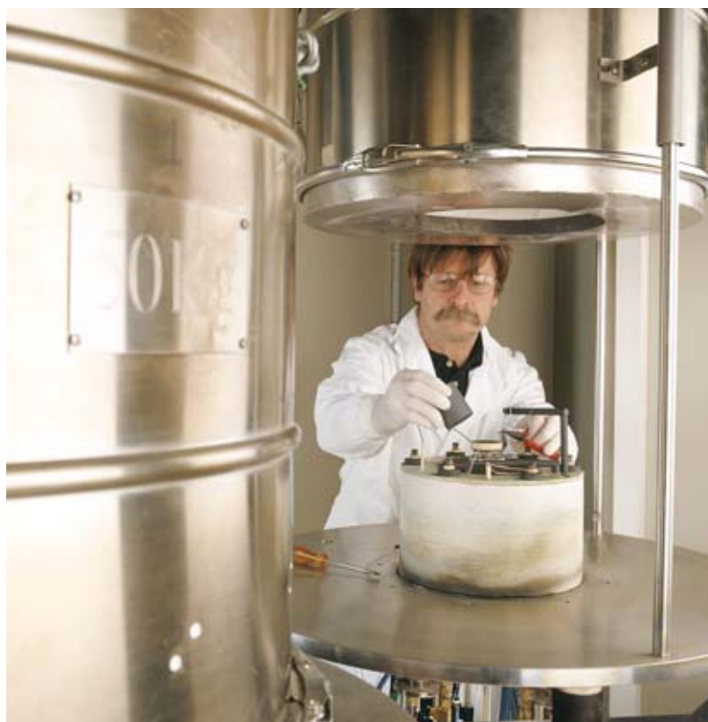
SOFC fuel cell being positioned on a test bench allowing determination of single-cell and stack voltage and current characteristics.
