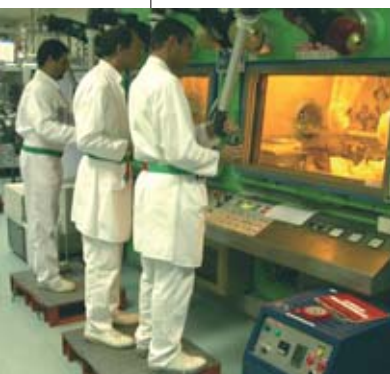
Fabrication laboratory for ceramic matrices developed for conditioning long-lived radionuclides.
