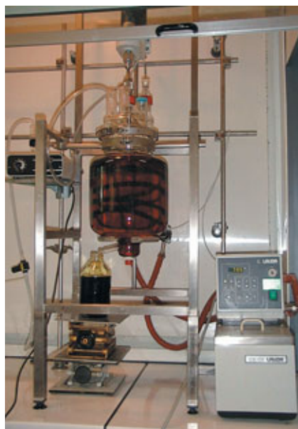
Reactor used at the CNRS/LMOPS for synthesis of the sulphonated polyimides used for the composition of high performance proton conductive membranes.
