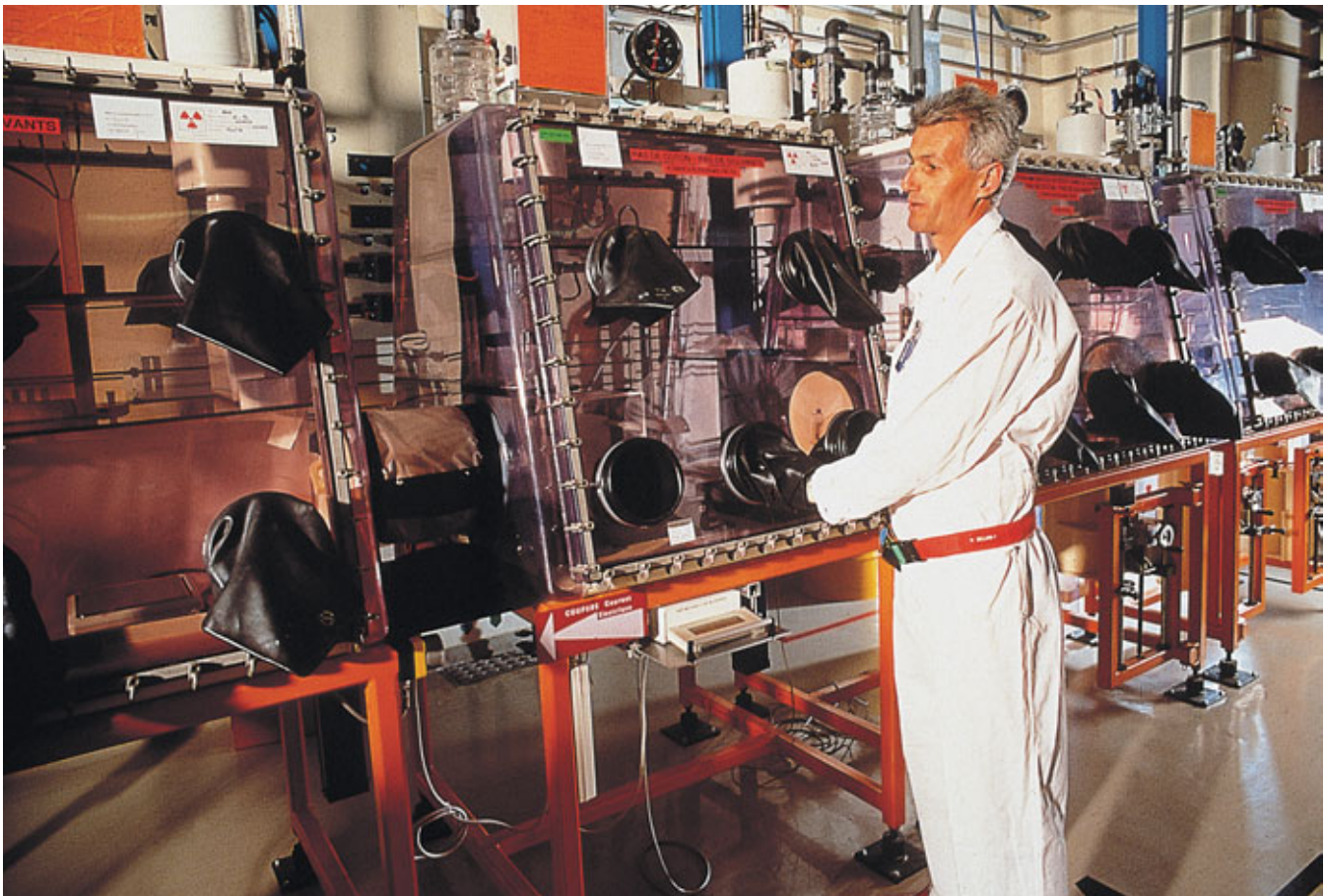
Glove box titration during MOX fuel handling.
