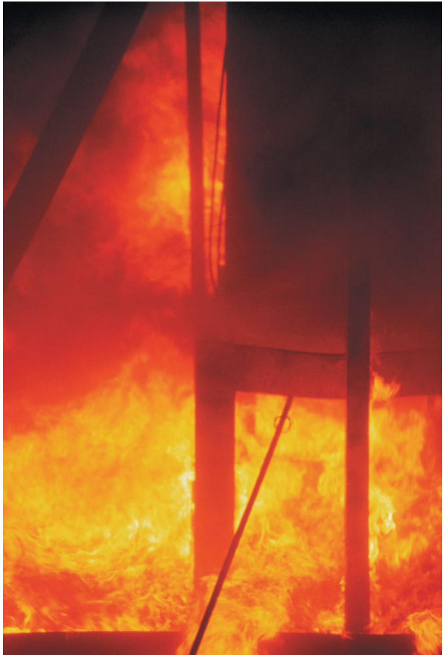
Fire resistance test of a plutonium shipping container.
