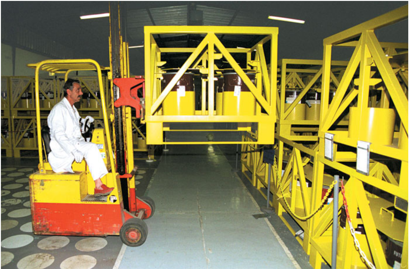
Handling non-irradiated fissile material at the CEA/Cadarache. The material is packed in drums and stored on centered cages to protect against the risk of criticality.
