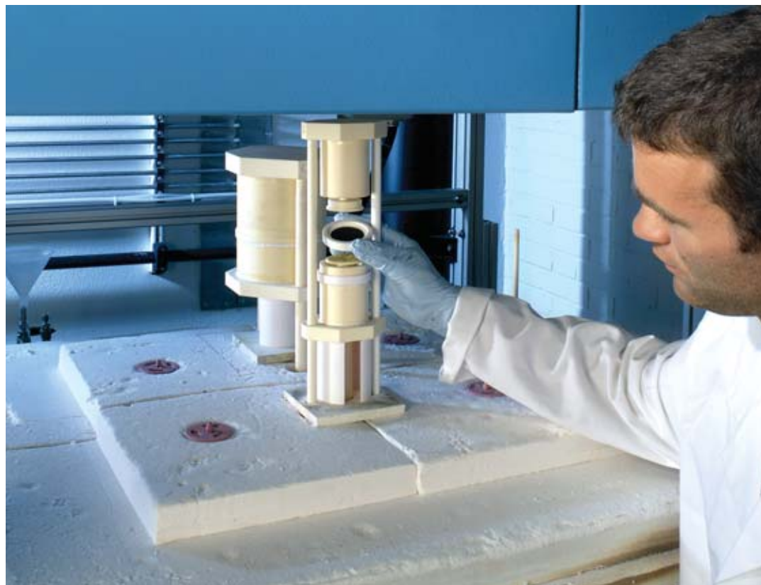
The Solo test rig, set up at the Grenoble Center, allows investigation of SOFCs with a variety of fuels, and serves as an aid to modeling for processes occurring at the anode.
