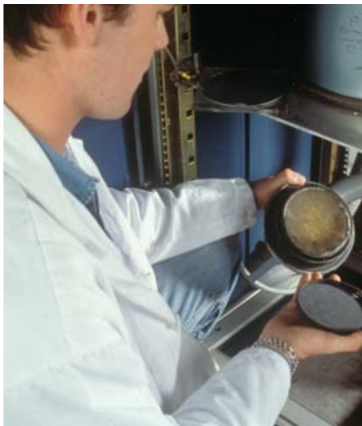
Measurement of physicochemical parameters of water in samples taken from the environment of a CEA centre. Inset: filter record corresponding to a weekly air sample before dispatch to nuclear analysis laboratory.
