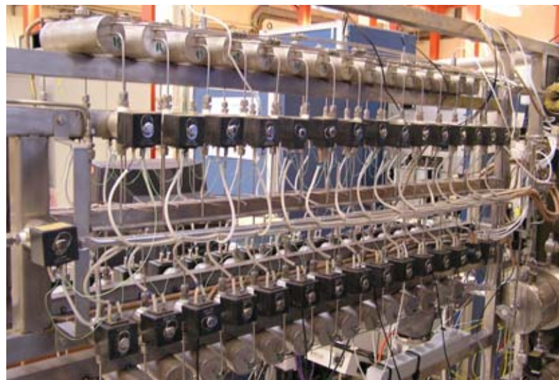
Gas-sampling system of the Mistra facility, at CEA/Saclay. Connected to a mass spectrometer, this allows mappings of concentration fields to be drawn up for the simulated hydrogen inside the vessel.
