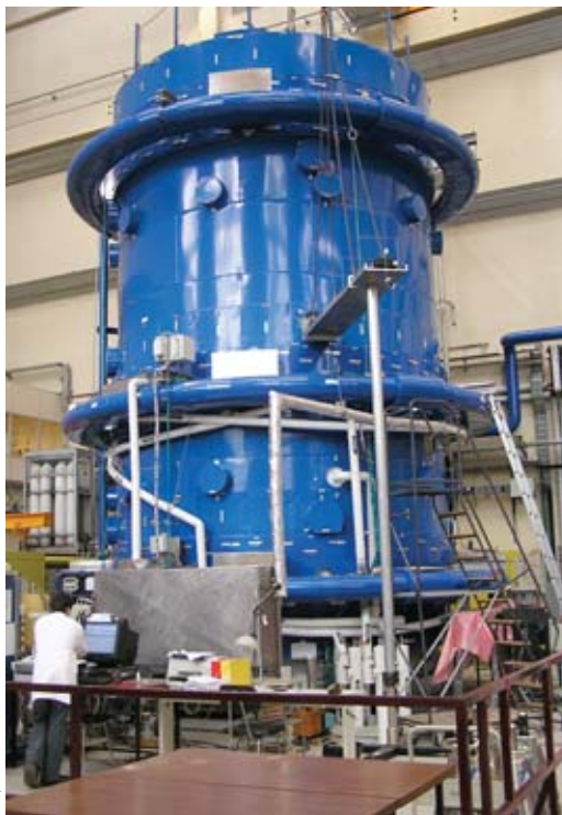
Mistra facility, at CEA/Saclay, for investigation of the release of hydrogen (experimentally simulated by helium) in a confined environment.
