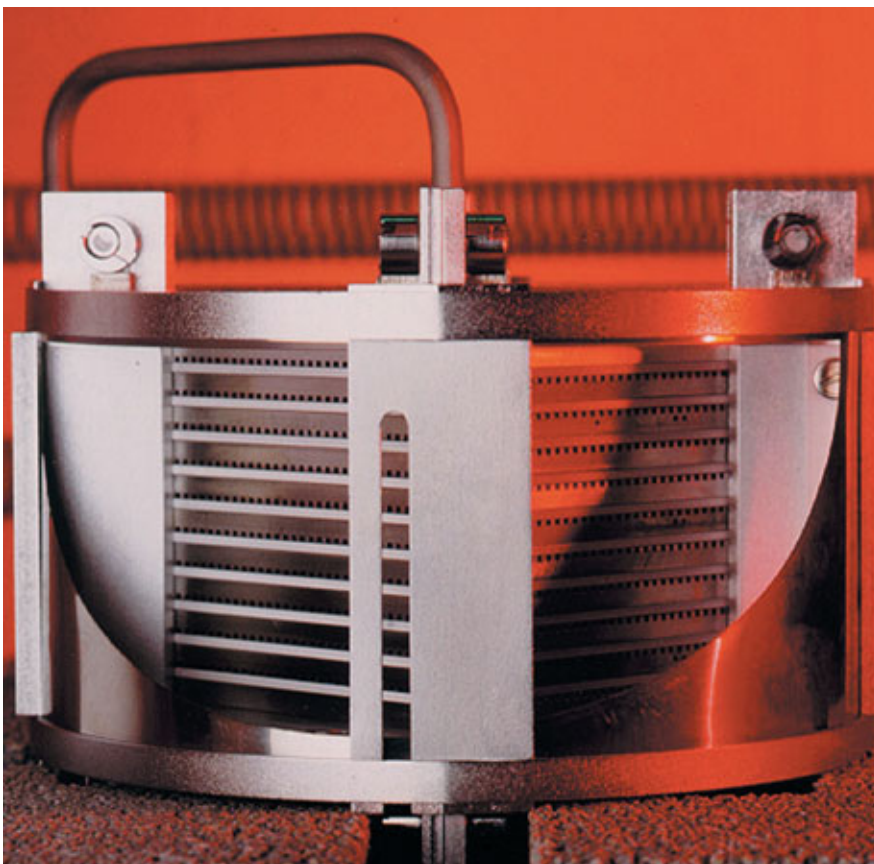
SOFC cell prototype developed at the Jülich research centre in Germany.
