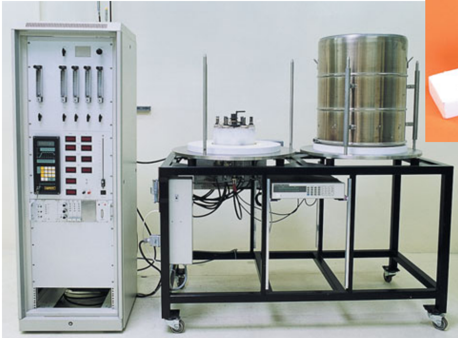
SOFC cell measurement bench. The cabinet is used to control the input of gas into the oven, and its temperature. The cell is inserted into the bell-shaped oven. Its voltage is measured according to the temperature, the intensity of the discharge and the gaseous environment.
