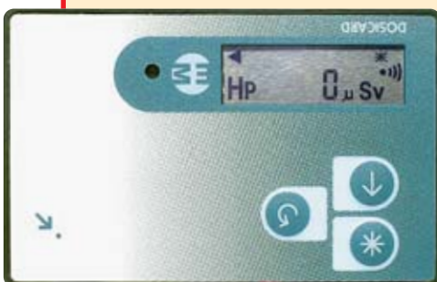
Dosicard dosimeter for real-time dosimetric monitoring.
