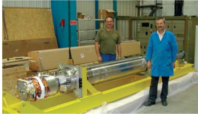
The MEGAPIE spallation target, built by ATEA in France, prior to delivery, in June 2005, to the Paul Scherrer Institute (PSI), in Switzerland. Out-of-beam tests are being carried out prior to the irradiation stage, scheduled for the first half of 2006.
