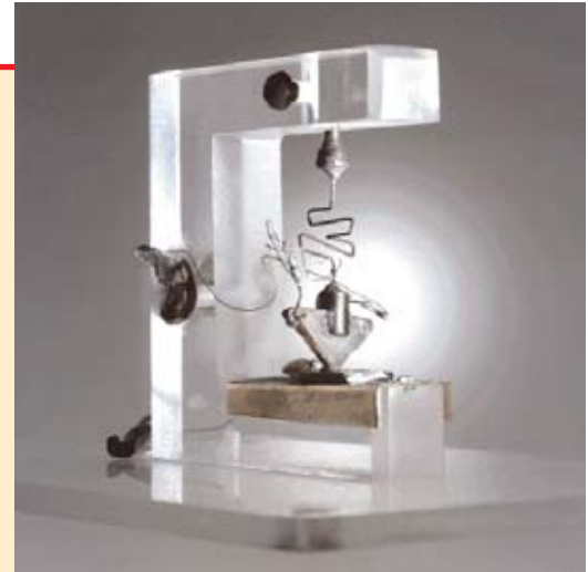
The very first transistor.
