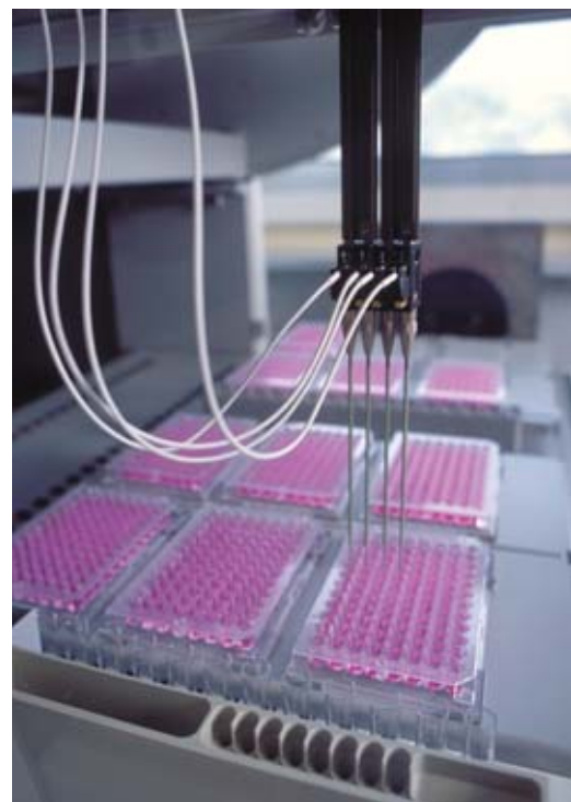
Pipetting-diluting robot used at the CEA Marcoule Centre to test antigen-antibody interactions simultaneously on a large number of micro-plates.
