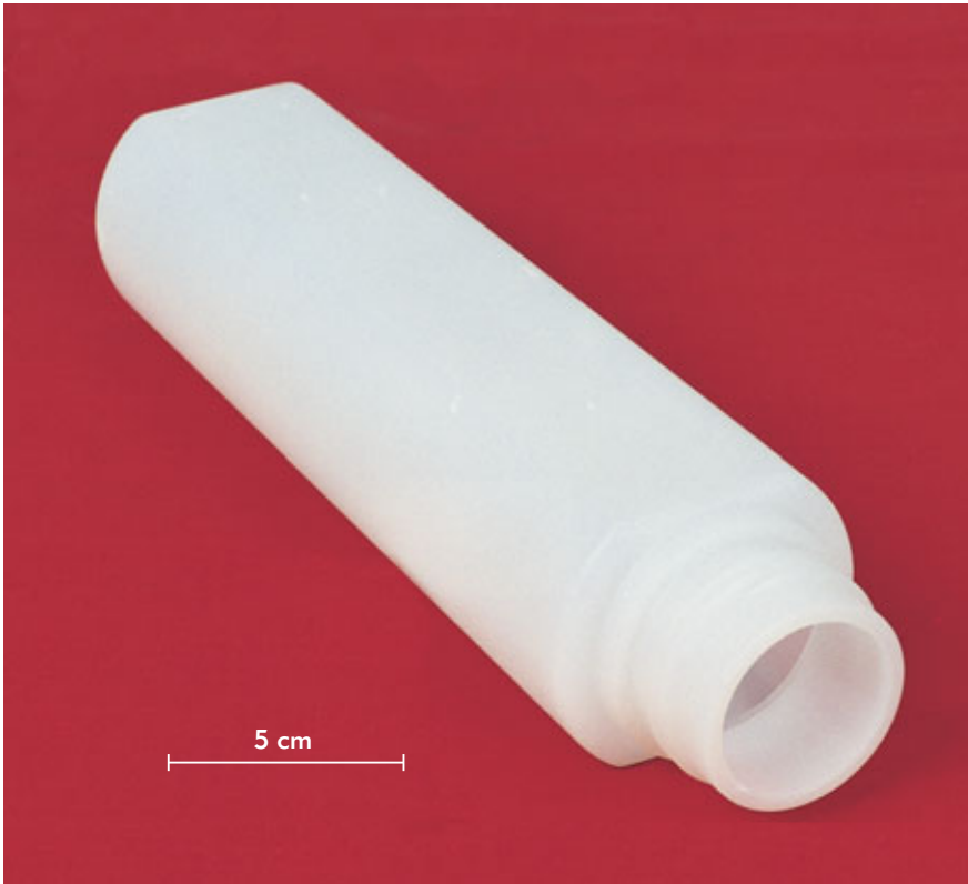
Prototype of a multi layer polymer tank, for hydrogen storage.
