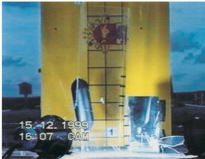
14 m drop test on a high pressure hydrogen tank at the CEA/Cesta's external testing ground.
