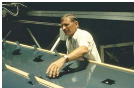
Double-walled roof model, allowing natural air currents to cool a dwelling's temperature, being tested in a solar simulator at CEA/Cadarache.
