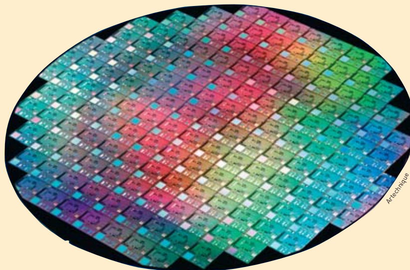
300-mm silicon wafer produced by the Crolles2 Alliance, an illustration of current capabilities using top-down microelectronics.
