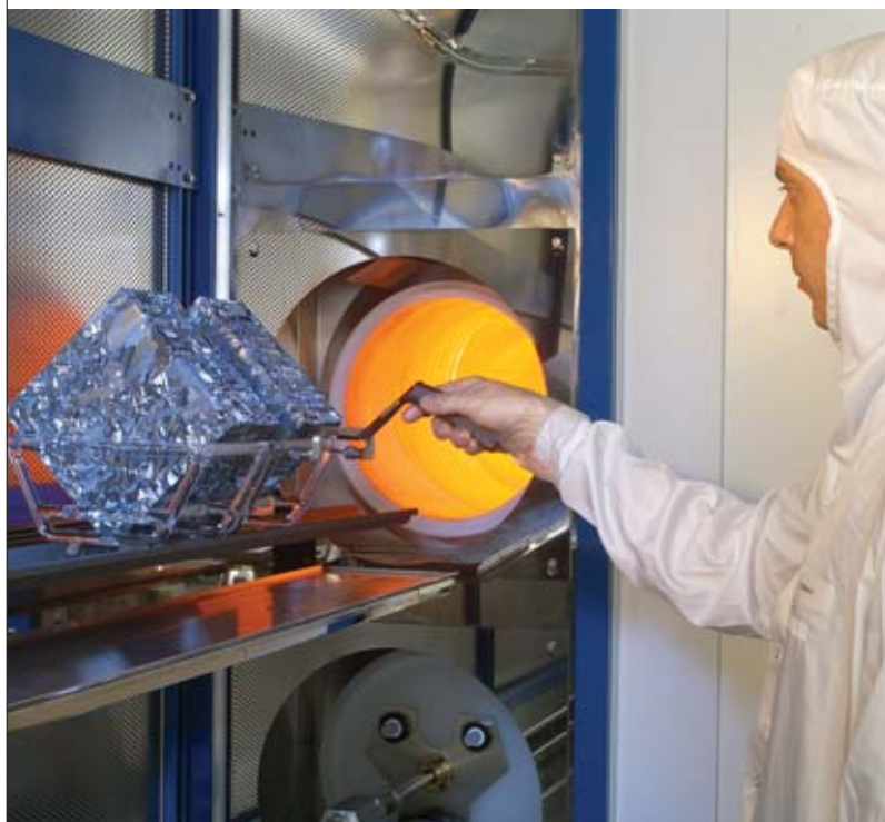
200-mm × 200-mm silicon wafers being loaded onto the source boat of the diffusion furnace used to form the photovoltaic cell's emitter. The Restaure Platform at CEA/Grenoble is one of the few to cater for such a wafer area, the standard being 150 mm × 150 mm.
