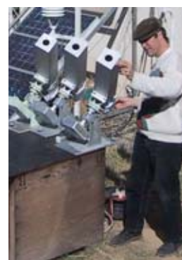
Calibration of pyranometers by a new method improving measurement accuracy. The three devices are collimators aimed at the Sun.
