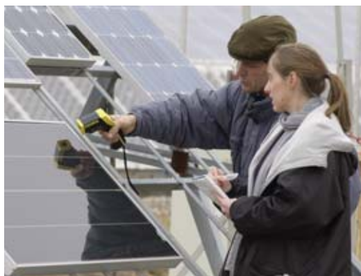
Measurement of the surface temperature of a photovoltaic solar module.
