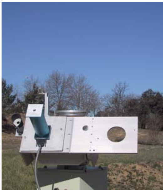
Absolute cavity radiometer, allowing highly precise measurement of solar flux intensity.
