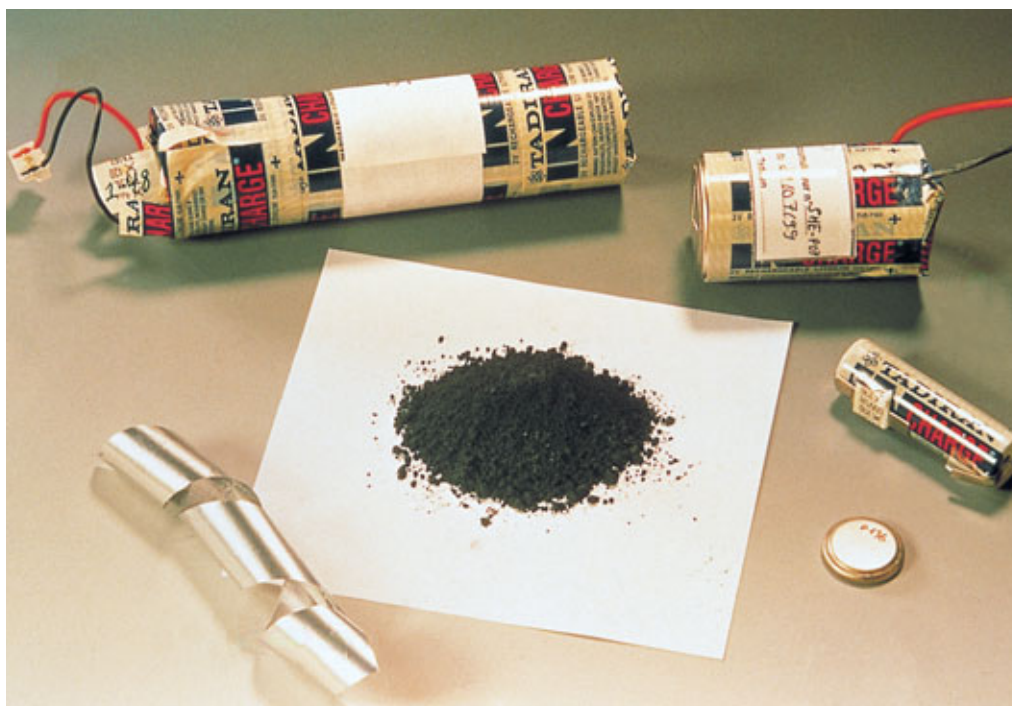
Different lithium storage battery prototypes. The button-type storage battery was manufactured at the CEA/Grenoble, whereas the cylindrical and spiral storage batteries were made by Tadiran Batteries Ltd., the CEA's Israeli partner. The positive electrode's active material (in powder form) was developed at the CEA.
