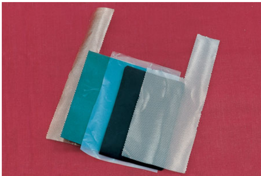
Components of a lithium-ion polymer battery: on each side the current collectors (copper and aluminium grids), the negative electrode (green), the positive electrode (black) and in the centre the electrolytic membrane. This membrane absorbs the electrolyte and so makes a polymer gel.
