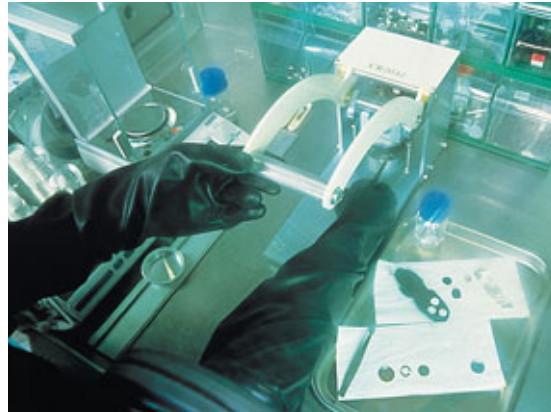
Assembling a lithium storage battery in an anhydrous glove box, with argon scanning, at the CEA/Grenoble.
