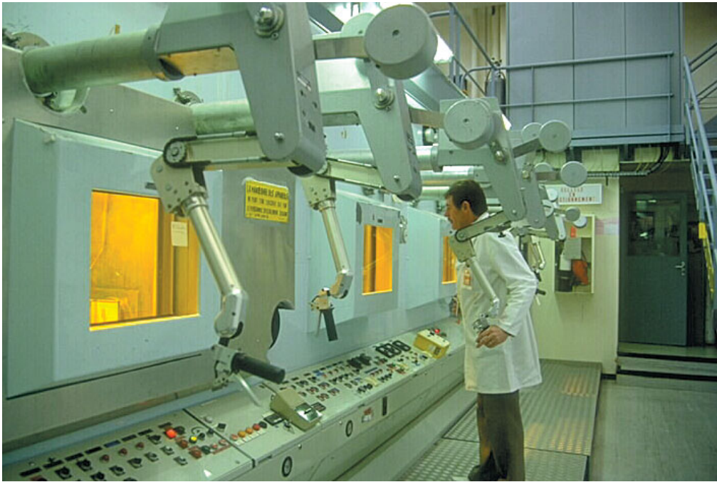
The CEA/Cadarache Comir unit where the physical properties of irradiated fuel samples are measured.
