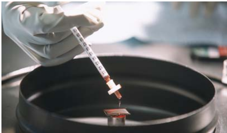
One of the fabrication steps for polymer photovoltaic cells: spin deposition of the photoactive polymer material.
