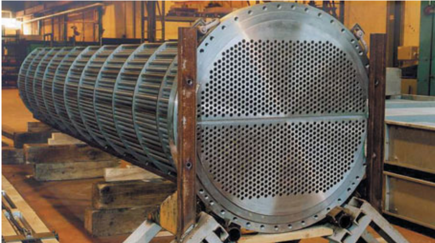
Heat exchanger with high-performance tubes being manufactured by CIAT, partner of CEA/GRETh.
