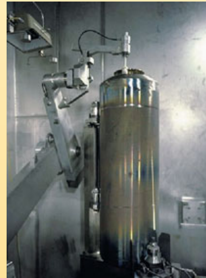
Vitrified waste canister being inspected in the R7 vitrification facility in the Cogema UP2-800 waste-reprocessing plant at La Hague (Manche département).
