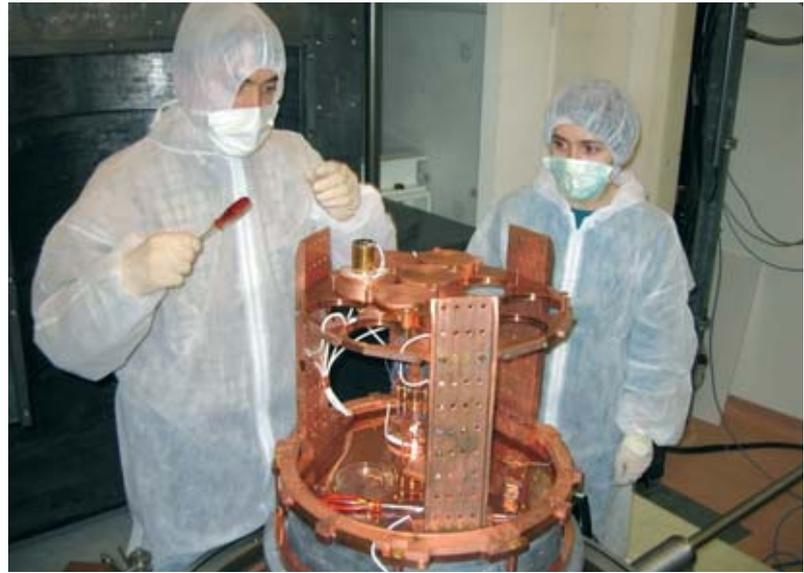
Positioning one of the ten 12-bolometer stages used in the EDELWEISS II experiment.
