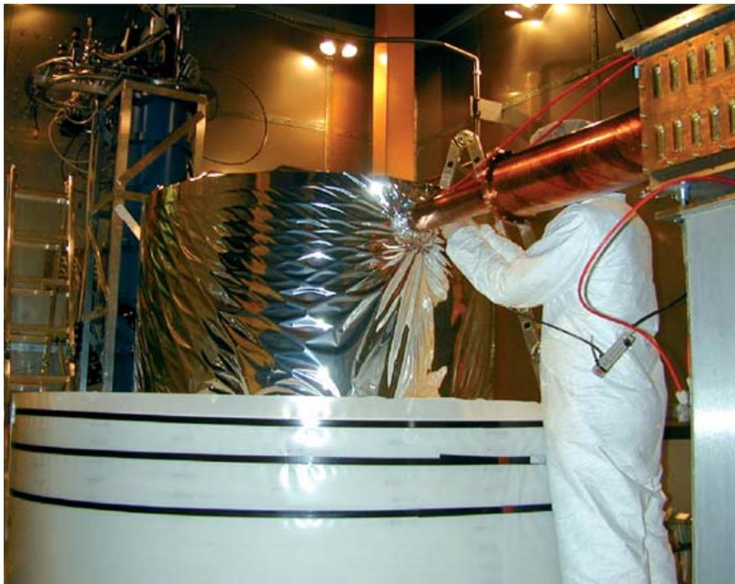
The refrigerator and cryostat for the CDMS experiment, installed at the Soudan Mine (Minnesota).
