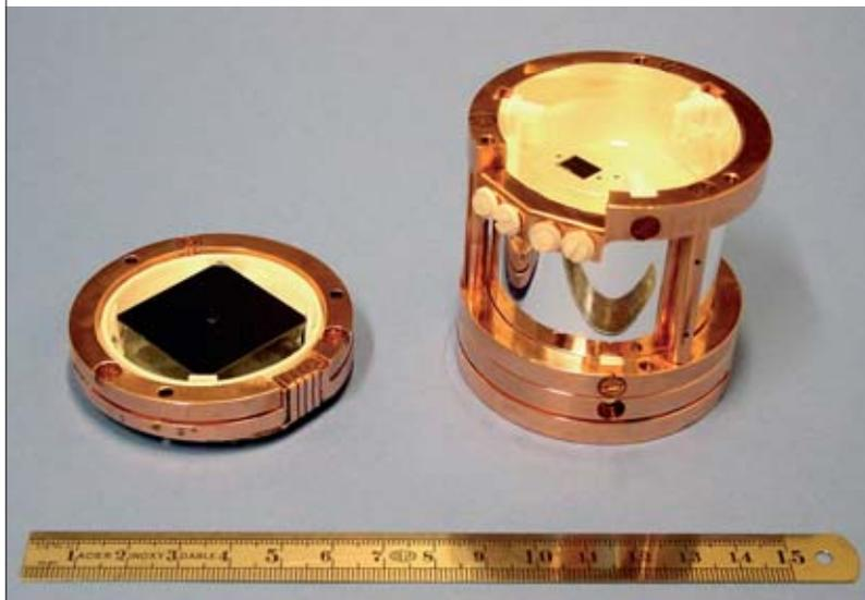
Prototype detector module for the CRESST II experiment.
