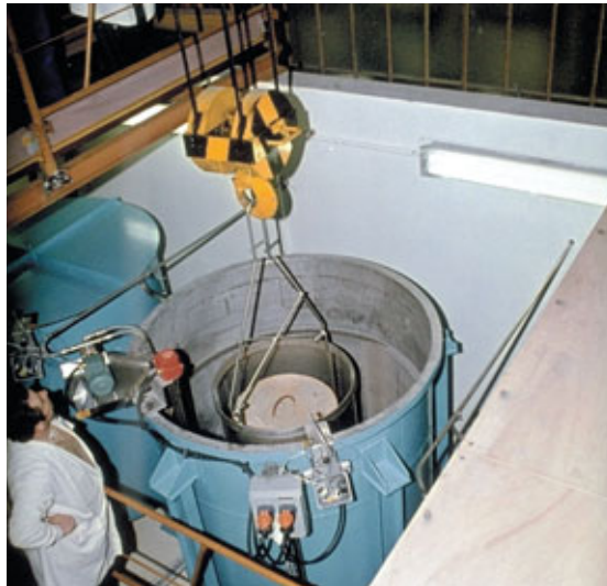
Waste package leaching research installation at CEA/Valrhô-Marcoule.
