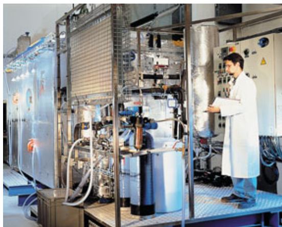
Mascilia experimental device at CEA/Cadarache, used for research into the long-term mechanical and hydromechanical behavior of the geomaterials confronted over time by a wide range of temperatures in high-level radioactive waste storage or disposal facilities.
