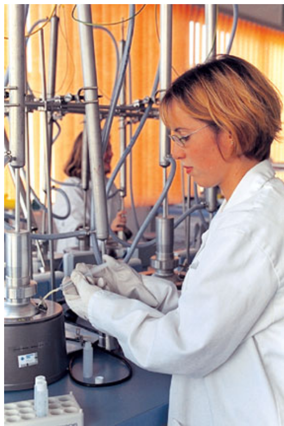
Sampling leachate on Soxhlet-type equipment to assess the concentrations of elements leached from a "nuclear waste" glass package.
