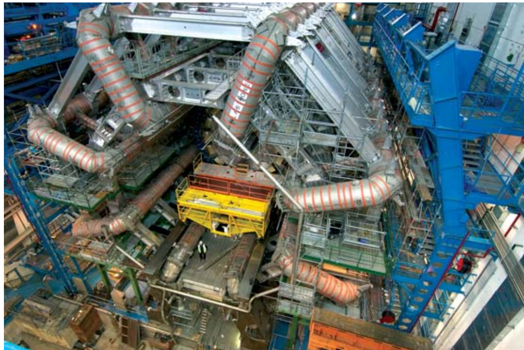
General view of the ATLAS (A Toroidal LHC ApparatuS) detector, with its eight toroidal magnets in place, in November 2005. After detecting its first cosmic rays in situ , in its hadronic calorimeter, ATLAS initiated operation of two of its tracking systems, in June 2006, to record such rays.
