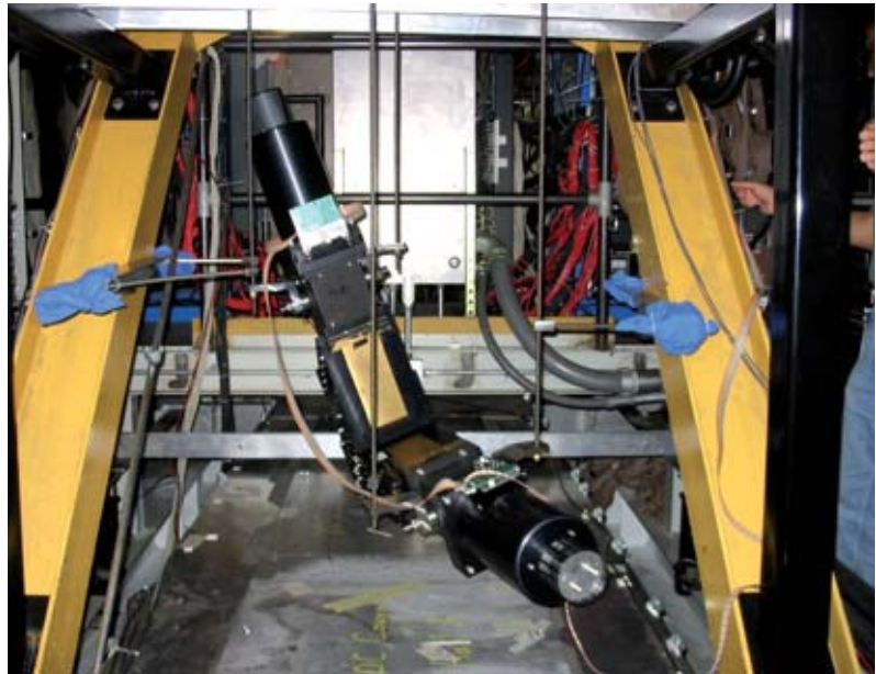
A detector for the HAPPEX experiment, set up at the exit of the magnetic spectrometer. The active component in the detector, a gold color in the photograph, is made up of alternating polished brass and silicon strips. The electron flux is intercepted by these strips, in which it produces a luminous signal, which is taken up by the silicon, and propagated to photomultipliers, which may be seen at either end.
