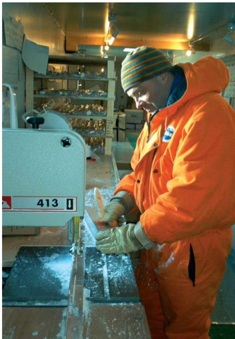
Once ice cores are extracted, samples are cut and prepared for subsequent analysis, in Europe. Many analyses are also effected on an ongoing basis, on the ground.
