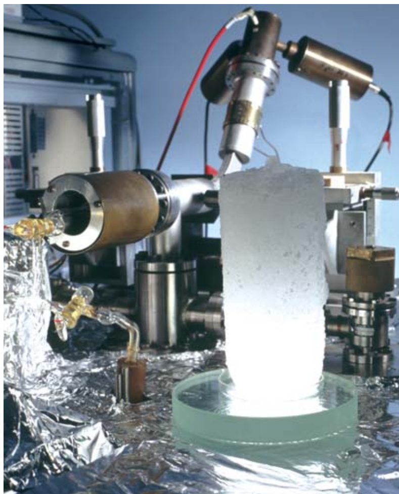
Analysis of an ice core, using a mass spectrometer. Measurements of ice deuterium and oxygen 18 content allow past temperature variations to be reconstructed.
