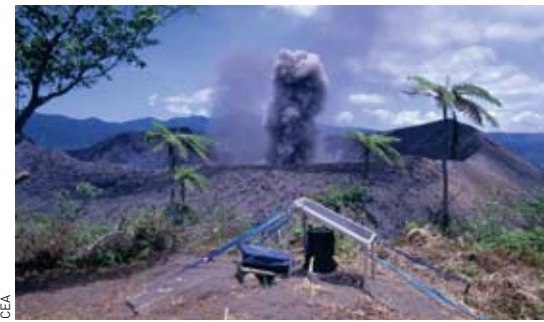
At left, map showing the location of infrasound station I22FR (shown at center), set up in New Caledonia, relative to the active volcanoes in Vanuatu, detected constantly at the station. Right, the Yasur volcano. A microbarometer is positioned at the mouth of the crater, to measure the very small pressure variations around atmospheric pressure, in the infrasound band.
