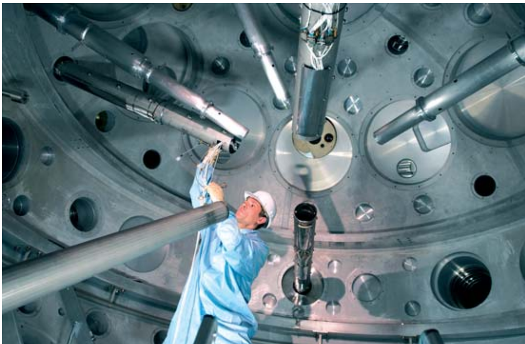
Checking diagnostics inside the Laser Integration Line (LIL) experiment chamber, the prototype installation for the Megajoule Laser (LMJ), consisting in one elementary laser line, comprising four beams
