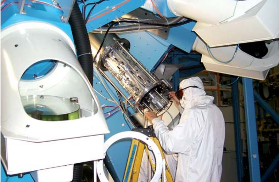
Wideband spectrometer, to measure hohlraum radiation temperature, fitted to the Omega installation at the University of Rochester (New York State), in the United States.
