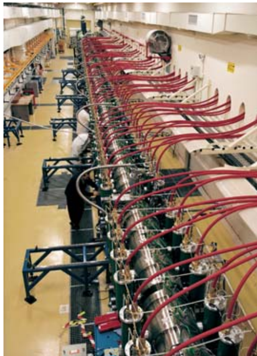
AIRIX accelerator hall. AIRIX (Accélérateur à induction deradiographie pour imagerie X: X-Ray Imaging Radiography Induction Accelerator) comprises 64 induction cells (to which high voltage is supplied via the red cables), bringing electron energy to 20 MeV
