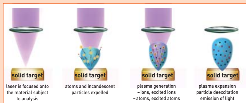
Figure a. Principle schematic of LIBS plasma generation.
