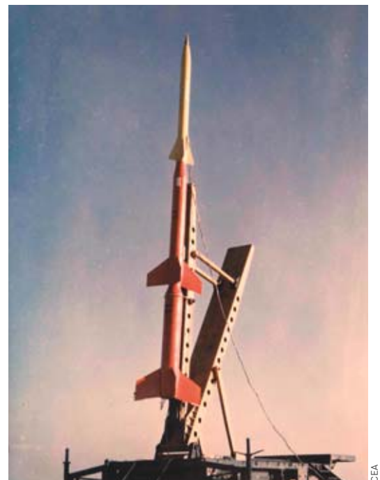
The first space experiment to be carried out by CEA, on 27 January 1959. A Geiger counter was mounted on board a converted missile, to effect one of the first measurements of gamma radiation from the sky.
