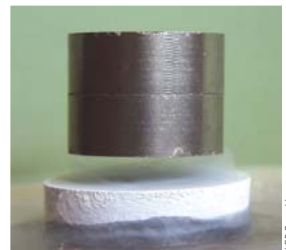
The discovery of high-critical-temperature superconductivity made it possible to see how superconductivity manifests in the open air in the form of a magnet floating above a pellet of liquid-nitrogen cooled YBaCuO, which is now a famous example of the effect.
