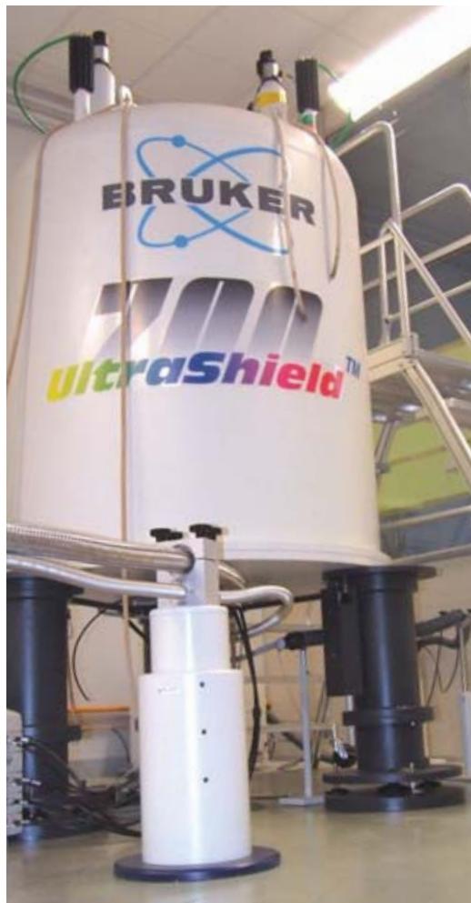
16.4-T NMR spectrometer magnet used to study three-dimensional protein structure. Inside this magnet, the hydrogen nuclei, i.e. protons, have a resonance frequency of 700 MHz.
