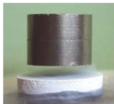
The discovery of high-critical-temperature superconductivity made it possible to see how superconductivity manifests in the open air in the form of a magnet floating above a pellet of liquid-nitrogen cooled YBaCuO, which is now a famous example of the effect.
